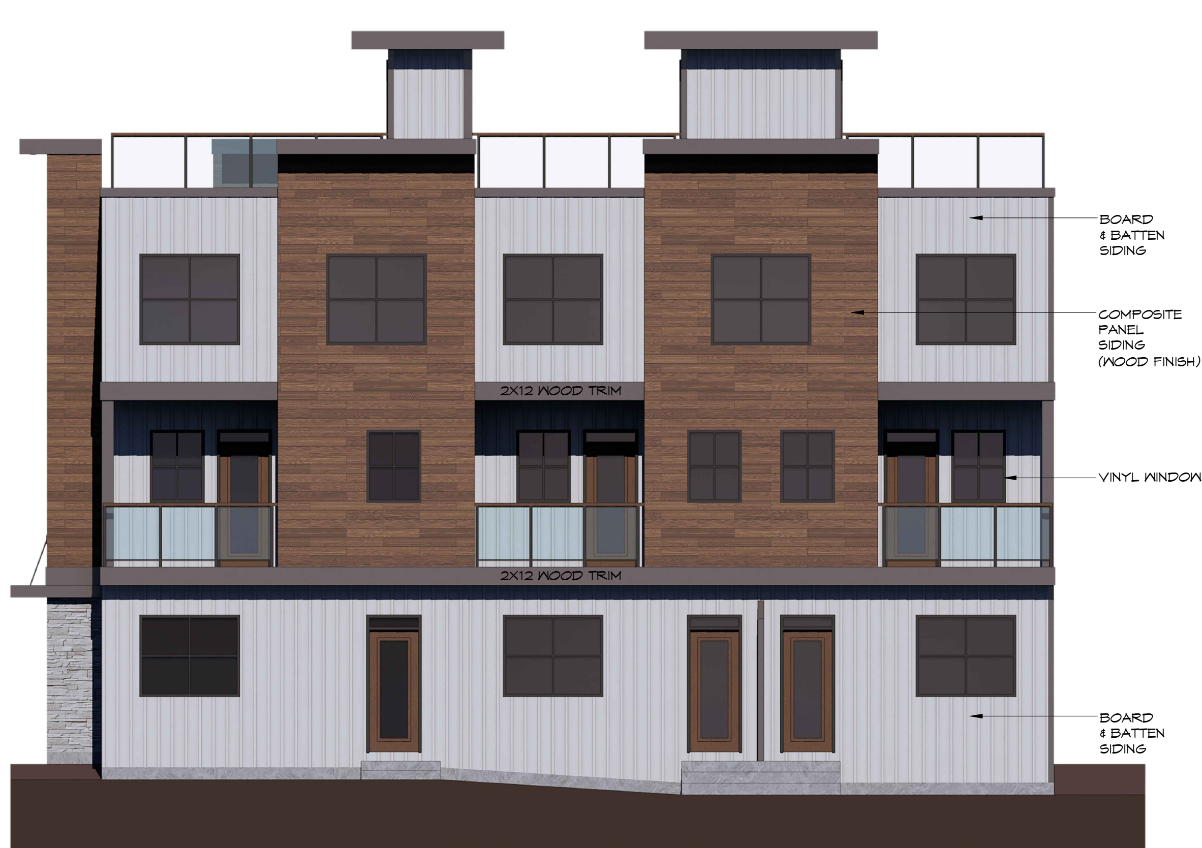
3 BUILDING #9 - REAR ELEVATION A-3.17 SCALE: 3/16" = 1'-0"
