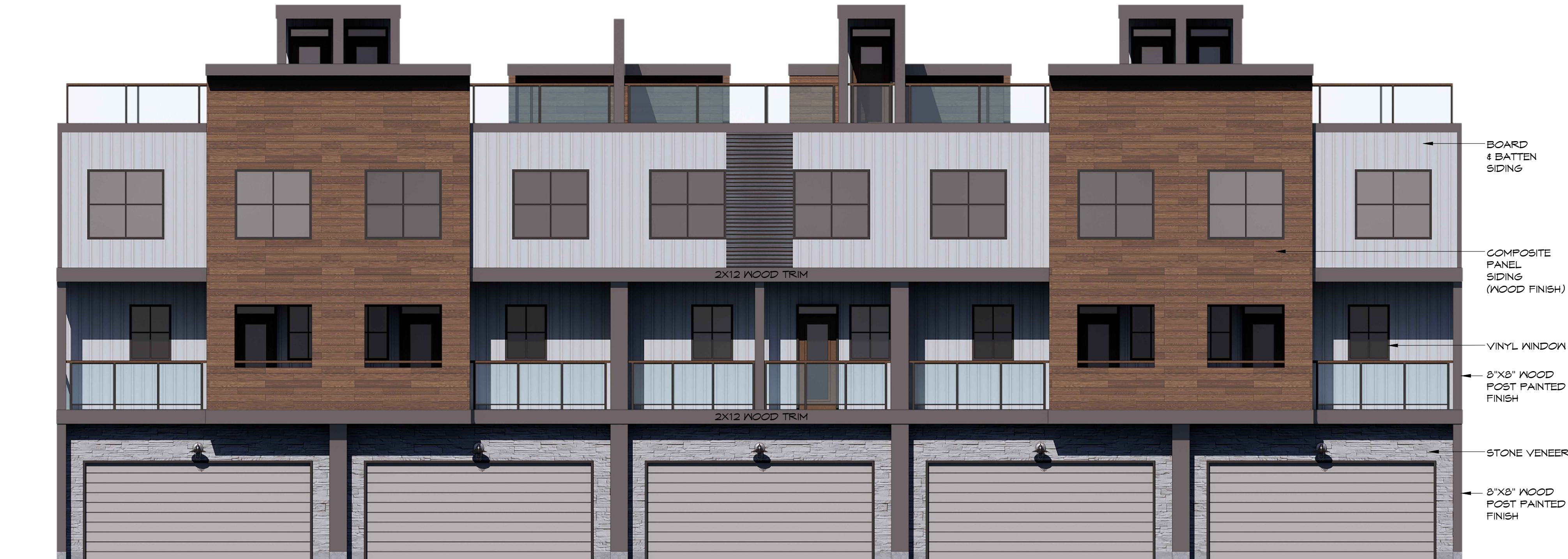
2 BUILDING #5 - REAR ELEVATION SCALE: 3/16" = 1'-0"
