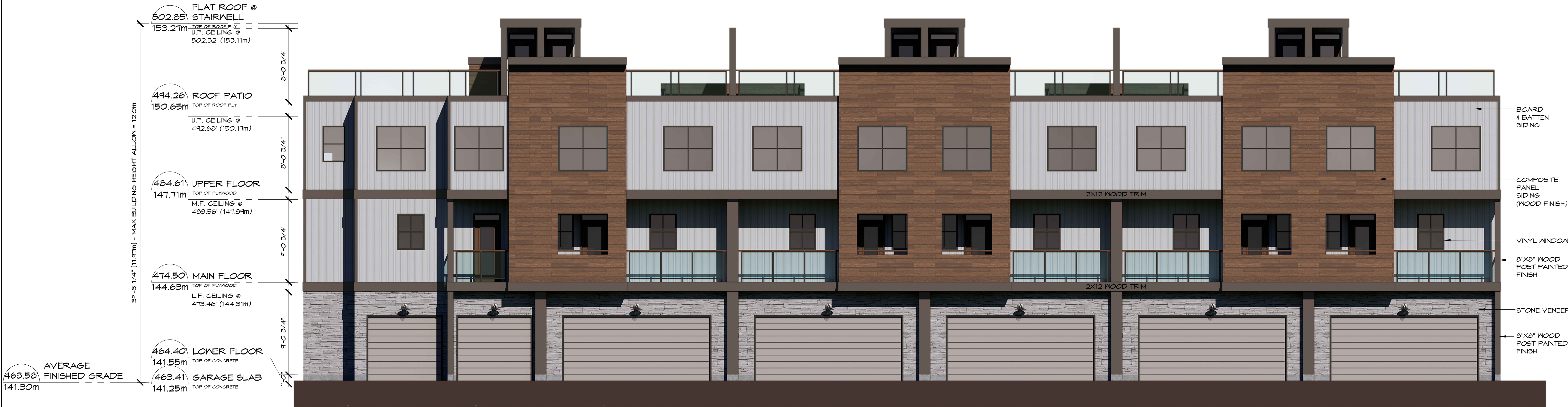
2 BUILDING #3 - REAR ELEVATION SCALE: 3/16" = 1'-0"
