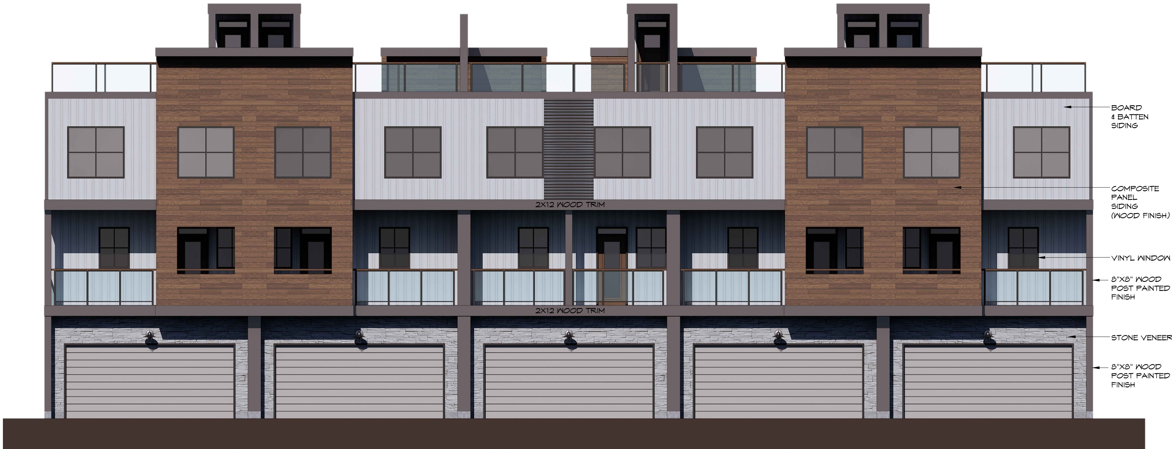
2 BUILDING #5 - REAR ELEVATION SCALE: 3/16" = 1'-0"
