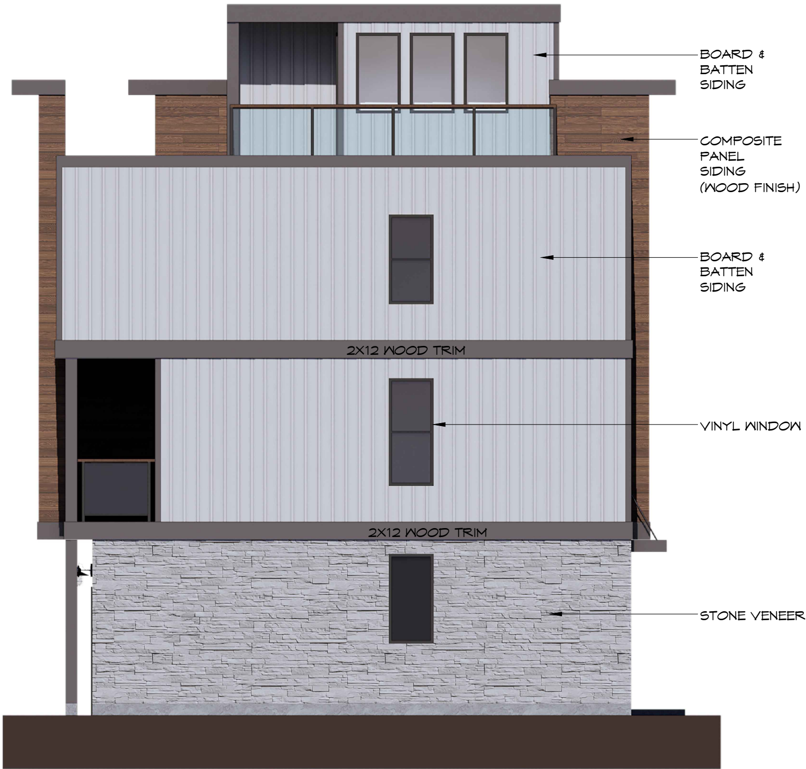
1 BUILDING #1 - LEFT ELEVATION SCALE: 3/16" = 1'-0"
