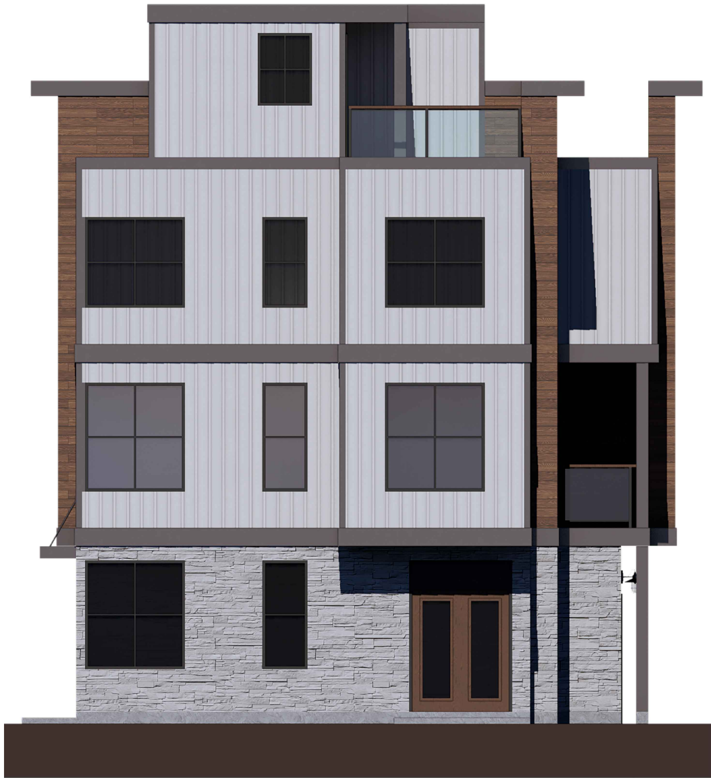
2 BUILDING #1 - RIGHT ELEVATION SCALE: 3/16" = 1'-0"
