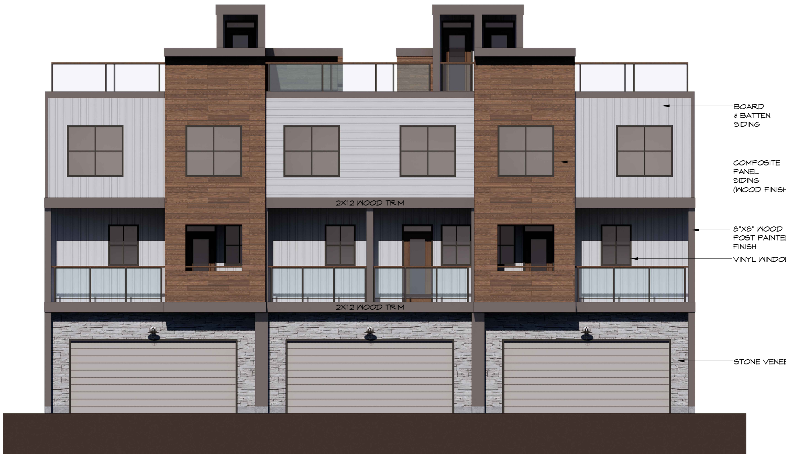
3 BUILDING #10 - REAR ELEVATION A-3.18 SCALE: 3/16" = 1'-0"
